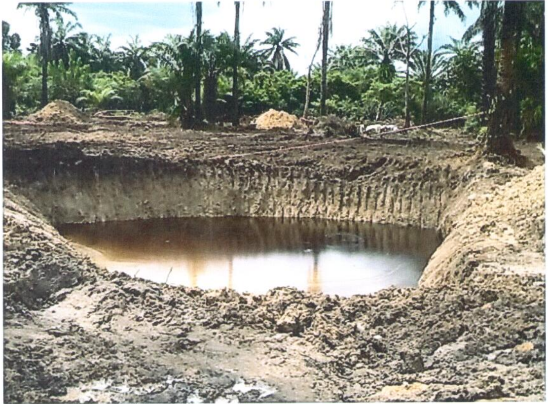
Plate 4: Free phase oil in the excavated pits
